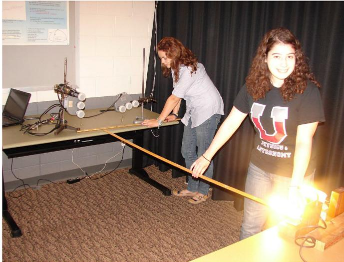
**Figure 2.** Union College students working with the VSRT. Two “triple” DirecTV feeds, taken from TV satellite dishes, used here as radio antennas, receive and detect the radio emission from compact fluorescent light bulbs (CFLs). Only one feed of each triple is active. The CFLs can be moved to assorted separation distances. The output spectrum from the interferometer is displayed on the laptop screen, and the data files are recorded.
