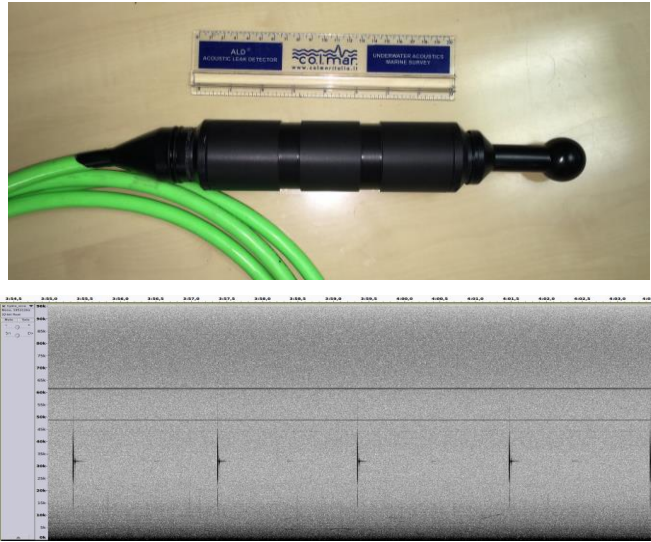
Figure 2. Top: An external hydrophone of KM3NeT, produced by Colmar Company (Italy). Hydrophones will be put on DU bases and, in the case of ARCA, also on Junction Boxes. Bottom: Spectrogram of about 10 seconds of data acquired by the hydrophone during operation of ORCA (Detection Unit 2). The signals of the LBL beacon (32 kHz) are clearly visible, dolphin’s whistles at about 5 kHz and another source (9 kHz) are also detected.
