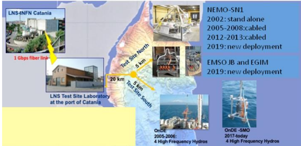
Figure 2. Configuration of the subsea infrastructure offshore Catania, where the EMSO Western Ionian Node is located (North Branch). Running and foreseen experiments are indicated.
