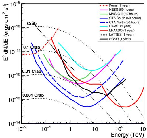
**Figure 1.** Differential sensitivity (multiplied by  $E^2$ ) to a Crab-like point gamma ray source of different experiments and projects. The best fit of the Crab Nebula data obtained by different detectors [17] is reported as a reference, extrapolated to 1 PeV
