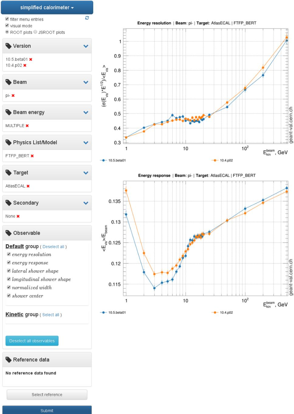
**Figure 2.** Plots of "simplified calorimeter" test results for Geant4 releases 10.5.beta01 and 10.4.p02 with 10.5.beta01 selected as "reference".
