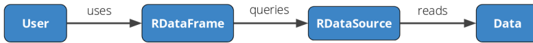
Figure 3. RDataFrame can read any columnar data format through a dedicated data source implementation. Expert users can implement and seamlessly integrate data sources for their format of choice.
