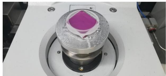
Fig. 4 Demonstrator element on MRF for form correction.
