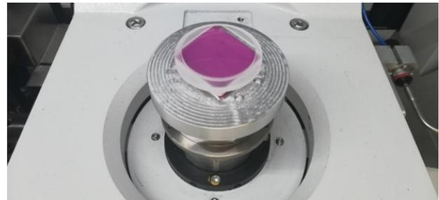
Fig. 4 Demonstrator element on MRF for form correction.
