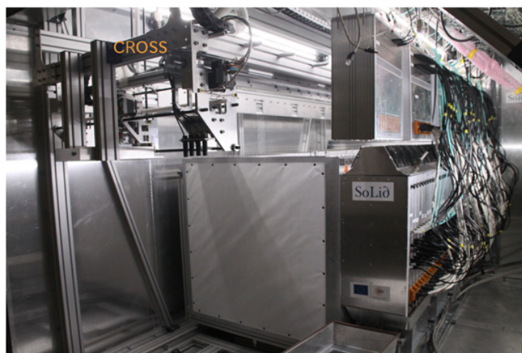
Figure 12. The detector, installed in the container. On the right, the module's service box, electronics and heat exchanger. The automated calibration robot CROSS can lower calibration sources between any modules.
