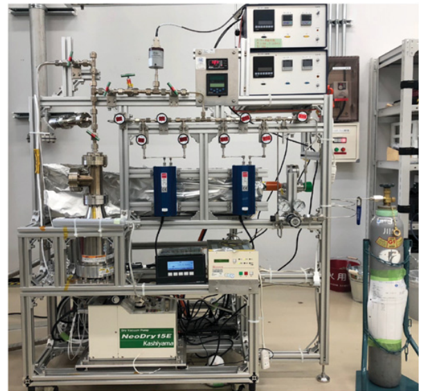
Figure 11. Vacuum system for confinement of ^3\text{He} and Rb in the glass cell of the spin filter.
