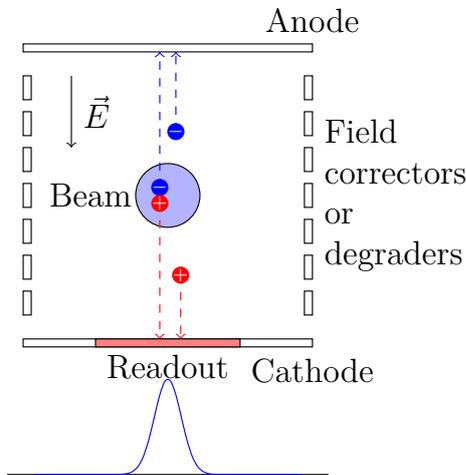
Fig. 2. Visual explanation of how an IPM works. The electric field between the electrodes can be reverted by inverting the polarity, giving the possibility to detect ions or electrons. Field correctors or degraders, left and right, improve the field uniformity.
