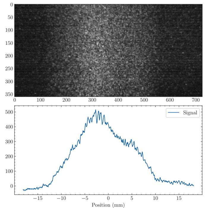
Fig. 12. Image of the beam profile at the lowest current and pulse duration possible at IPHI (0.5 mA, 50  $\mu$ s). In these conditions, the signal is close to the one expected at ESS for the worst case. Note that IPHI was not designed to work a such low current.
