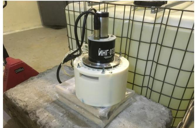
Fig.1 Experimental detector of FM in concrete structures.
