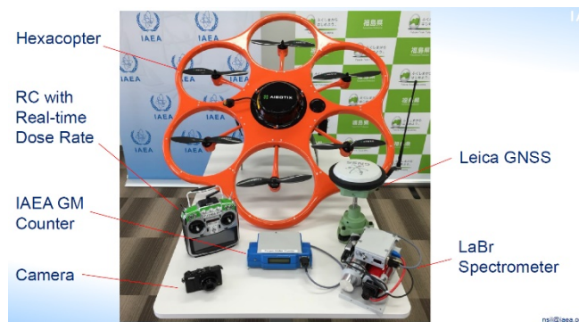
Fig. 2. Set of equipment provided to Japan, it includes two types of detection systems, based on GM and LaBr+PMT detectors. The RC of the UAV exhibits a real time dose rate reading.
