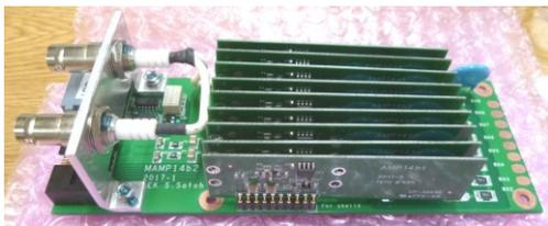
**Fig. 2.** PSD amplifier board.
