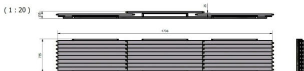
Figure 3. The MCORD modules consist of three sections, eight scintillators each.
