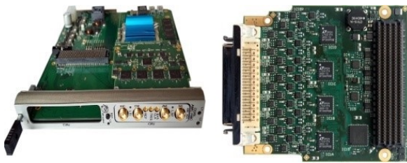
Figure 7. The separated electronic PCBs with for SiPMs, amplifier and power supply.
