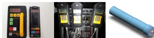
Figure 2. Left: EKO-C and EKO-D dosimetry probe. [6]. Center: Gamma-Scout dosimetry probe. Right: UM-EGM wide range gamma probe. [7, 8]
