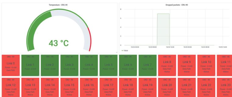
**Fig. 4.** Status of single CRU readout card: temperature, dropped packets and status of its 24 links
