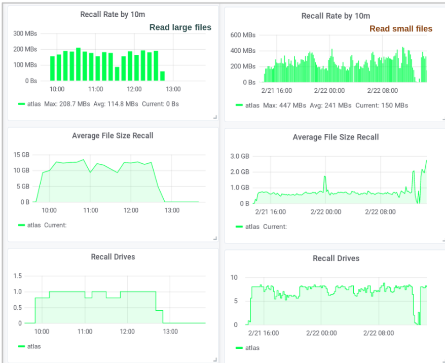
Figure 7: Reading small (less than 1.0GB file size) and large (larger than 9.0GB file size) files from tapes
