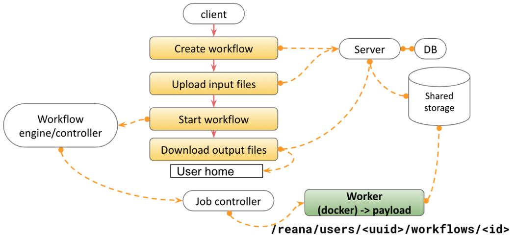
**Figure 3.** Schematic showing the REANA client creating a new workflow, uploading the necessary input files to a shared file system and running the payload inside docker containers.
