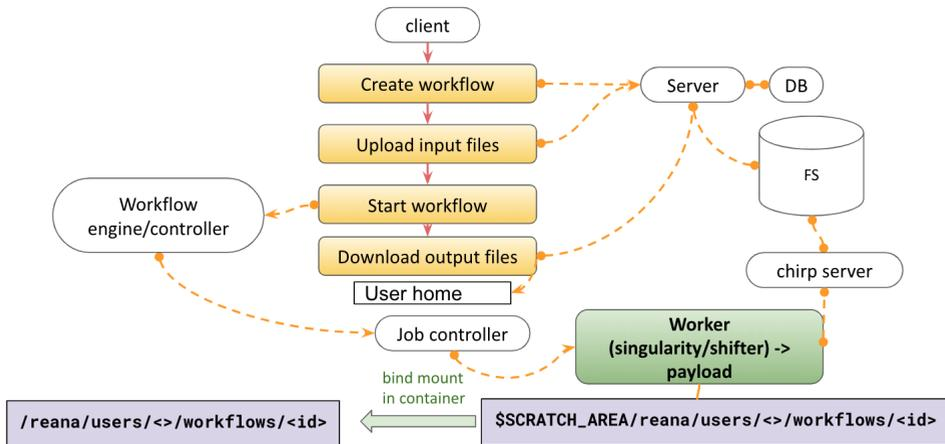
**Figure 7.** Schematic showing the REANA client creating and running new workflow, after integrating the detection and usage of HPC friendly container technologies and connecting the edge service file system used by REANA server via chirp and parrot
