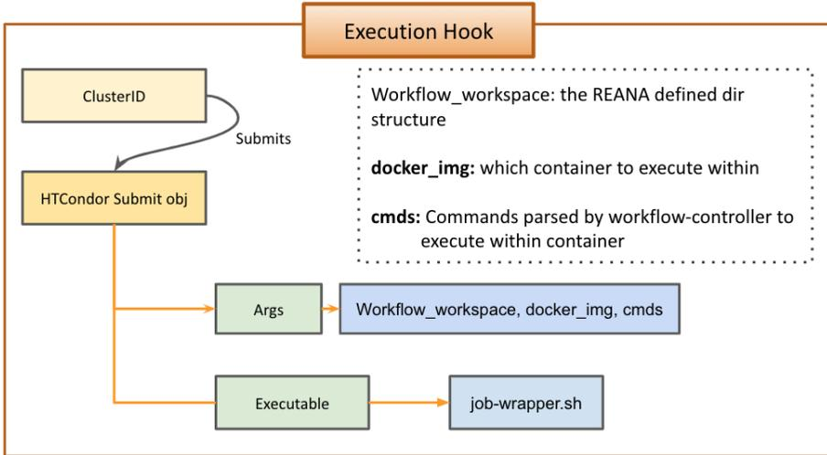
**Figure 4.** Job submit object creation and definition of arguments: workflow space absolute path, docker images and the commands to be executed
