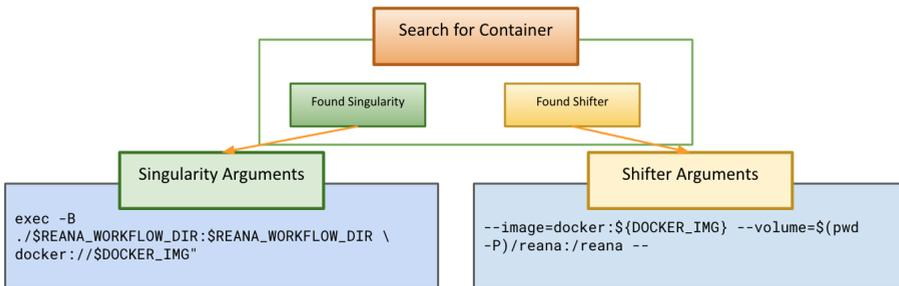
**Figure 5.** Detection of container technology available in the HPC worker and definition of parameters for it
