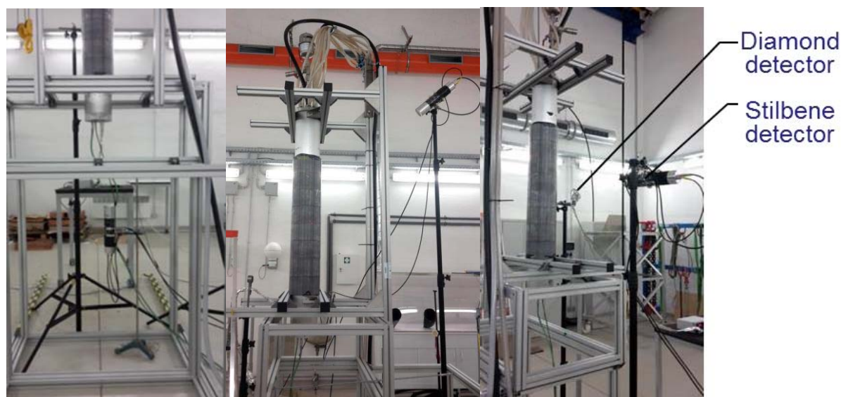
Figure 3. NG with a stilbene detector and a diamond detector placed in several measurement positions.
