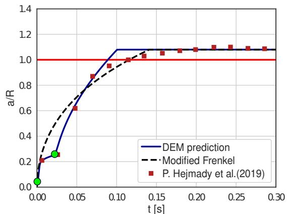
**Figure 4.** sintering curve of Polystyrene particles,  $R = 30.0 \mu\text{m}$  compared with Frenkel's model (dashed line), and experimental data (boxes) [4].
