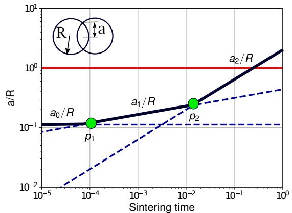
**Figure 2.** Regime map for three different sintering mechanisms. First, an adhesive equilibrium is modelled before point  $p_1$ , following the JKR flat zone. From point  $p_1$  to point  $p_2$ , it is defined the starting point at which the instantaneous compliance of the material takes place, and after point  $p_2$ , the material is sufficiently relaxed to flow under surface tension.
