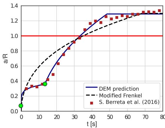
**Figure 6.** Sintering curve of PEEK 450PF particles,  $R = 25.0 \mu\text{m}$  compared with Frenkel's model (dashed line), and experimental data (boxes) [5].
