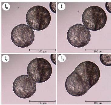
**Figure 3.** Snapshots from binary coalescence experiments with PA12 particles at different times,  $t_0 = 0.0$  ( $a/R$ ): contact point,  $t_1 : 0.1$  ( $a/R$ ),  $t_2 = 0.2$  ( $a/R$ ),  $t_3 = 0.8$  ( $a/R$ ).
