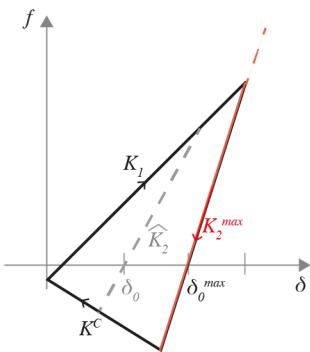
**Figure 1.** Visco-elasto-plastic contact Law. If  $\delta_0 > \delta_0^{max}$  the overlap enters to the "complete melting" of the particles.
