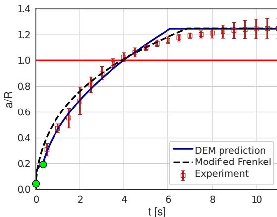
**Figure 5.** Sintering curve of PA12 particles,  $R = 31.5 \mu\text{m}$  compared with Frenkel's model (dashed line), and experimental data (boxes).
