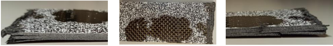
Fig. 9. Damage patterns of CFRP specimen at 113m/s a) Delamination b) Erosion c) Matrix Breakage
