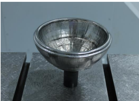
Fig. 1. WAAM Ta hemishell with conventional Ta rod at pole.
