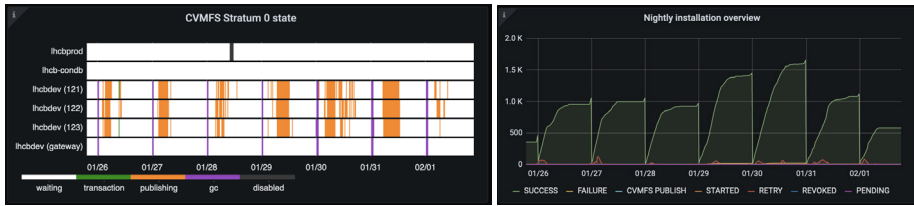
Figure 4. Extract from the Grafana dashboard for monitoring LHCb’s CVMFS installations with the server status (left) and the total number of installation tasks (right).
