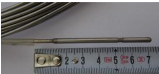
Fig. 1. CEA Cadarache manufactured miniature fission chamber.
