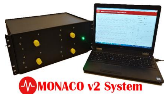
Fig. 2. CEA developed MONACOv2 acquisition system for fission chambers.
