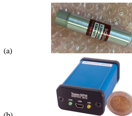
Figure 2 – (a) Ø10 mm x 9.5 mm CeBr 3 scintillator detector, with PM6660-SiPM and built-in preamplifier commercialised by Scionix. (b) Topaz-SiPM digital MCA module commercialised by BrightSpec NV.
