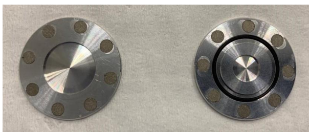
Fig. 1. The two halves of the coin target (24 mm diameter, 2 mm thick).
