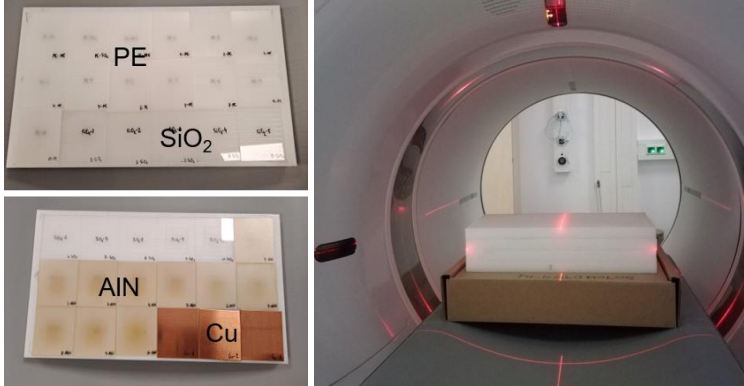
Figure 3. PET/CT measurement of the irradiated foils embedded between polyethylene plates.
