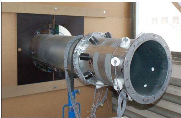
Fig. 1. Test prototype of ultrasonic flowmeter placed in 4Jtech laboratory, connected to an aerodynamic line.
