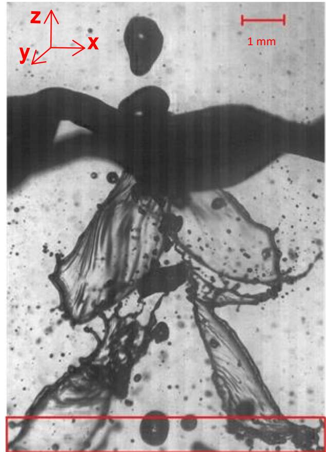
Fig. 6. The liquid dispersion on the crossing of two wires, We_d = 2217 and zero velocity of the air counterflow.
