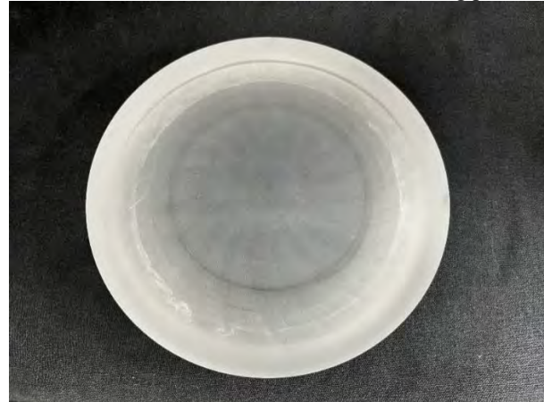
Figure 3 Sample of diameter 167 mm polished to the V-shape.
