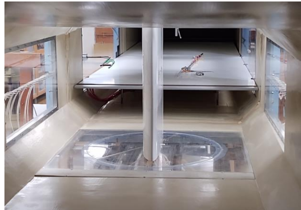
Fig. 2. Front view on the model (placed vertically) inside the test-section of the windtunnel.
