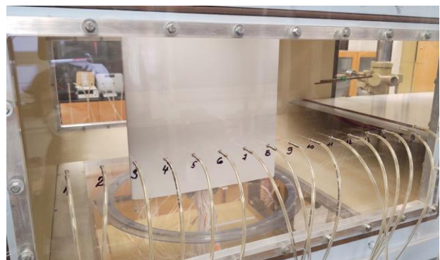
Fig. 3. Side view on the model (placed vertically) inside the test-section of the windtunnel.
