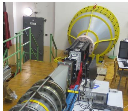
Figure 1. Test section mounted in the wind tunnel.
