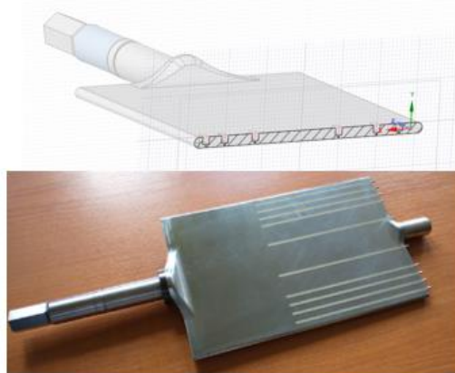
Figure 3. Static pressure probes mounted in the blades.
