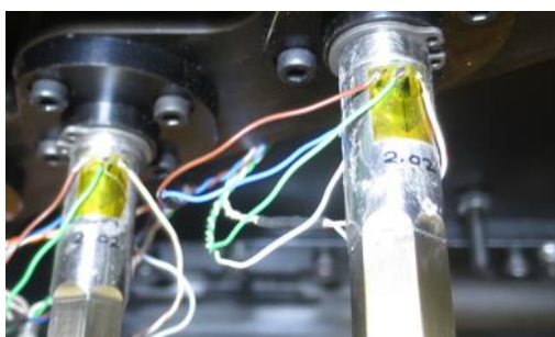
Figure 4. Strain gauge bridges mounted on blades No. 3 and 4.
