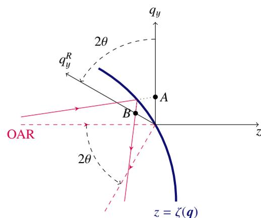
**Figure 1.** The reflection operator maps the point  $A$  of the incoming ray to the point  $B$  of the outgoing ray in the rotated coordinate system. The OAR (dashed) is mapped from the origin to itself. The incidence angle of the OAR on the reflector is equal to  $\theta$ .
