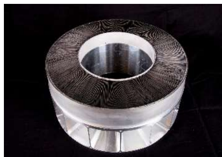
Fig. 2. A photo of a prototype WAVES device for selection of the final wavelength of the neutrons scattered at the sample position.
