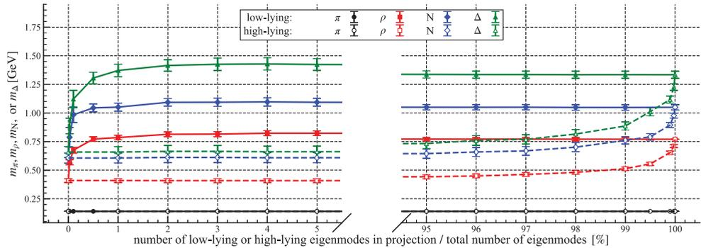
**Figure 3.** Hadron masses under the eigenmode projection in GeV unit plotted against the number of low-lying or high-lying FP eigenmodes in the projection. Pion mass  $m_\pi = 0.14\text{GeV}$  is used to set the physical hopping parameter for each measurement. The lattice spacing  $a = 0.1051(15)\text{fm}$  is used to set the scale. The solid and dashed lines are connecting adjacent data points for visibility.
