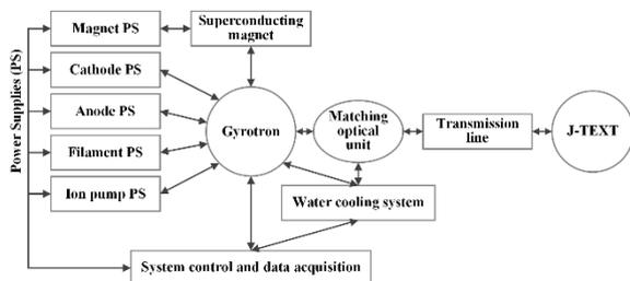
**Fig. 2.** Diagram of gyrotron operation platform.
