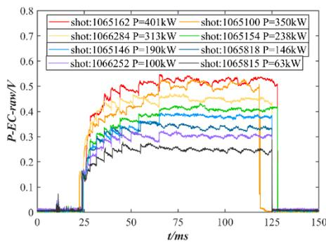
**Fig. 6.** Measured RF signal during gyrotron operation. Different shot has different power, therefore the RF signal has different value.
