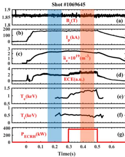
**Fig. 9.** Time evolution of plasma parameters for shot 1069645: (a) toroidal field  $B_t$ ; (b) plasma current  $I_p$ ; (c) line-averaged electron density  $\bar{n}_e$ ; (d) electron temperature at  $r/a = 0.72$  by ECE (no calibration); (e)-(f) the core of plasma electron and ion temperature obtained by XICS; (g) the ECRH power [14].
