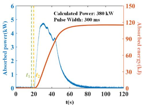
**Fig. 7.** A typical temperature rise curve during gyrotron operation, the left axis represents the power absorbed by water and the right axis represents the absorbed energy. Calculated power is 380 kW and the pulse width is 300 ms.  $t_1$  is the microwave injection time while  $t_2$  is the temperature rising time.
