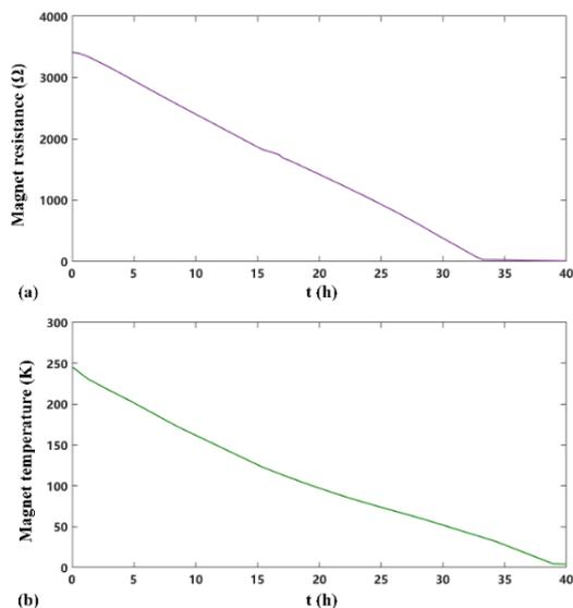
**Fig. 3.** Magnet resistance change (a) and magnet temperature change (b) during the cooling down process.
