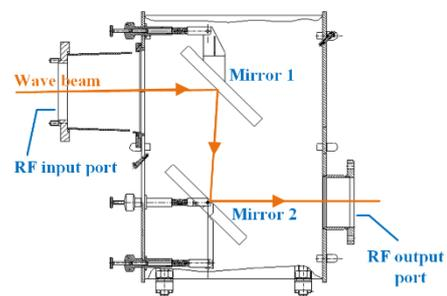
**Fig. 5.** Internal structure of MOU.
