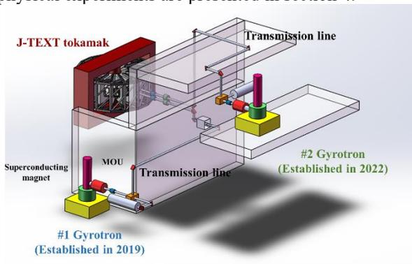
**Fig. 1.** Layout of J-TEXT 1 MW ECRH system
