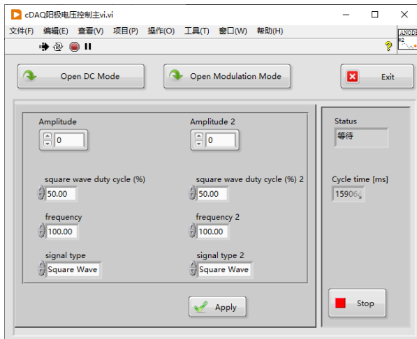
Fig. 6. The host computer control interface (modulation mode) of the ASIPP anode power supply.
