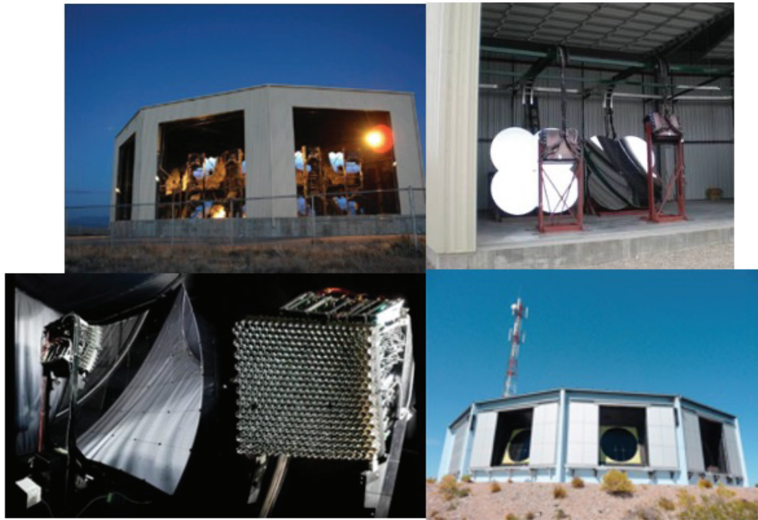
Figure 10. [Top L] BR air-fluorescence detector station for TA, [Top R] Middle Drum detector station for TA; Bottom [L] Auger mirror and pmt array [R] Auger detector housing.
