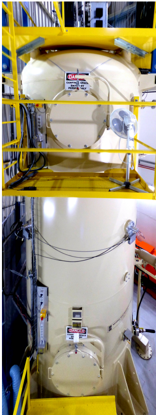
Figure 1. Picture of the vertical tank of the tandem accelerator of the MONNET facility.
