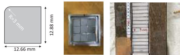
Fig. 4. The sample plate geometry of 233 U (left), the sample plates in the Al case (center), the case installed into the special fuel element “S” (right).
