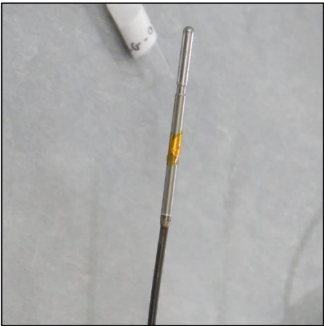
Figure 2: In-core fission chamber and gold foil dosimeter for power calibration.
