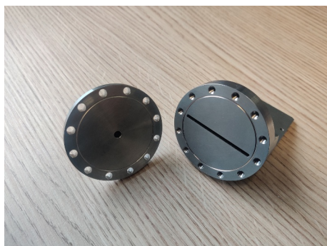
Figure 5. The Inconel 625 cell developed at ISIS to facilitate measurements of liquid NaOH at elevated temperatures.
