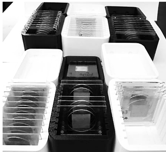
Fig. 6. Forty-two thallium foils mounted to frames and packaged to be sent to customers.
