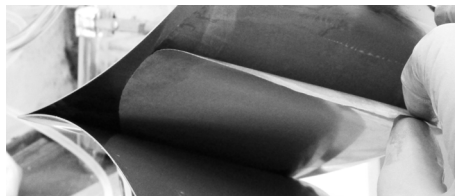
Fig. 4. Thallium foil, rolled in a stainless-steel rolling pack.
