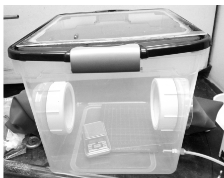
Fig. 2. Argon shower box with glove inserts.
