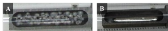
Fig. 3. Thallium in the tube furnace [A] as shot, before melting, and [B] as an ingot.
