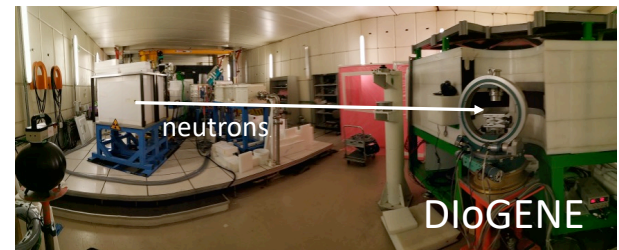
Fig. 7. The IPHI – Neutron facility: the accelerator in the back, the TMR + shielding box (white) with one small extraction hole and the DIoGENE instrument.
