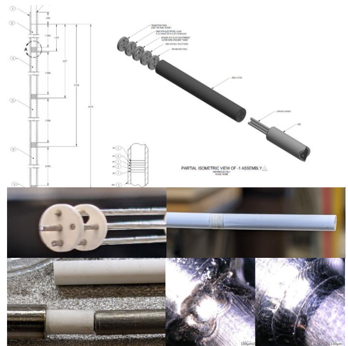
Fig. 7. MPFD arrays were constructed with 4 measurement locations separated by silica insulation and encapsulated in an Inconel sheath.
