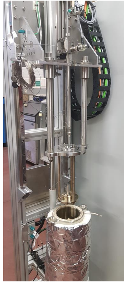
Fig. 12. High temperature LVDT calibration system.
