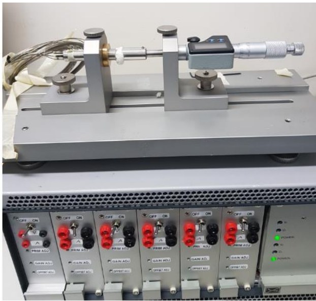
Fig. 6. Electronic units and calibration unit (on top) with mounted LVDT.
