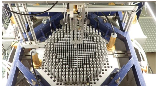
Fig. 3. View of PISTIL inserted in the central channel the CROCUS reactor.
