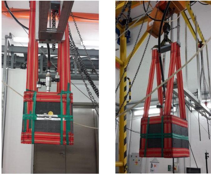
Fig. 3. Measuring the neutron leakage spectra in special laboratory [3]
