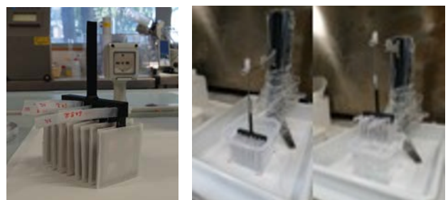
Fig. 3. set of samples in the fork (left) and immersion in the radioactive aqueous solutions. See text for details.
