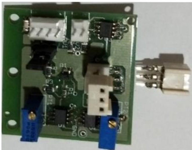
Fig. 2. PCB assembled to connect T_1 , T_2 and the IA circuit. T_2 connector, which is not shielded from radiation, is positioned outside the PCB area. The output signal, V_{dif} , can be evaluated by a typical multimeter or directly recorded in a microcontroller to be displayed on a small LCD screen.
